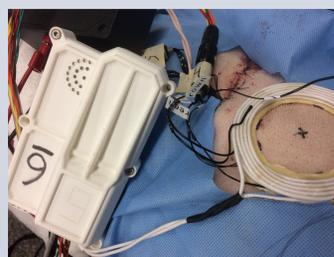
Implanted system with external coil and controller
