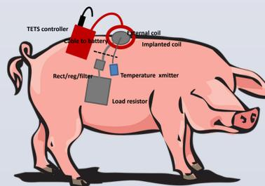
Placement of components for *in-vivo* testing
