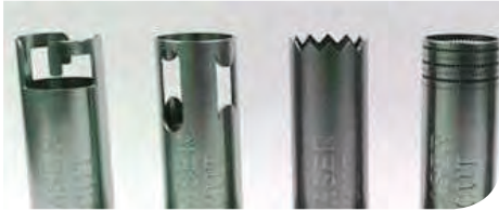
The four tubes show the unusual and complex features capable with a laser-Swiss machine.
